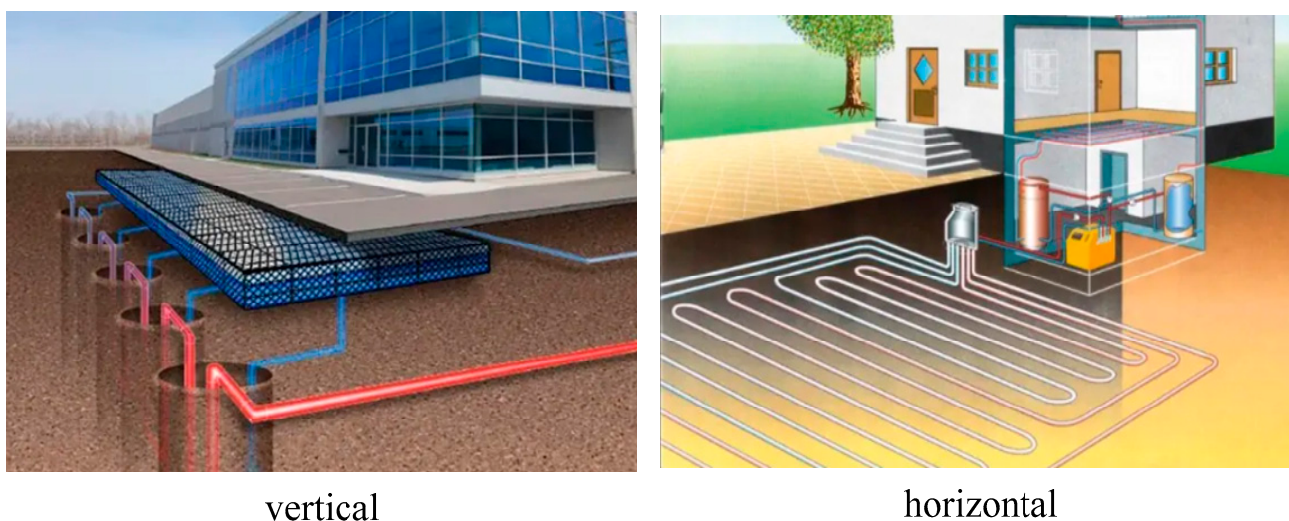
Figure 5. Principles of Two Geoenergy Resources Heat Pumps.
